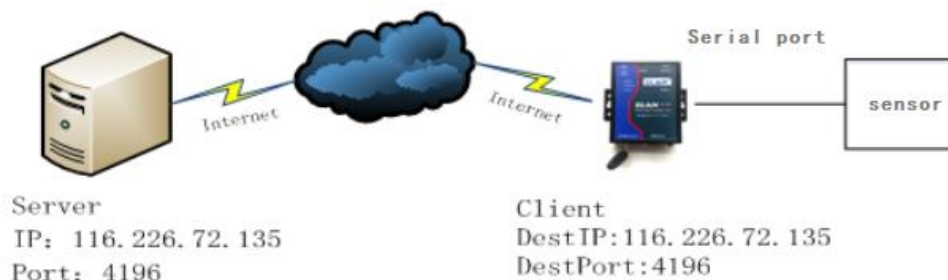
Figure 33 Networking structure diagram
